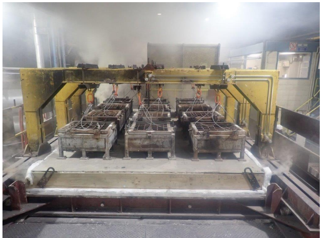
The unexposed face of the floor assembly after 34 minutes of testing
